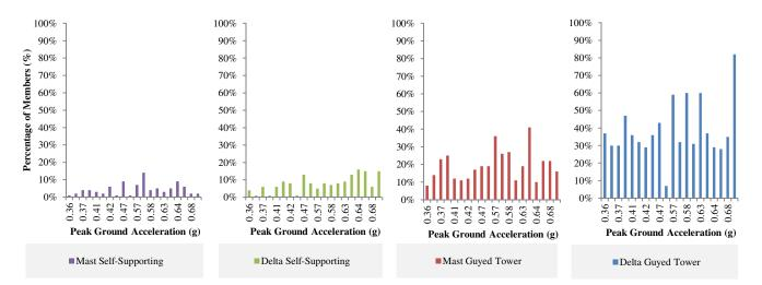
Figure 4. Percentage of members with seismic axial forces greater than those resulted from governing design load cases.
