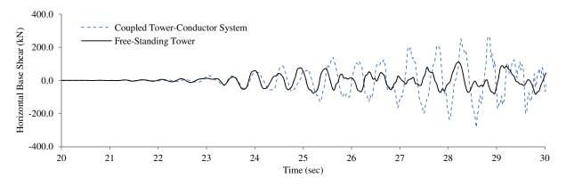
Figure 1: Time-history of horizontal base shear of Free-Standing Delta Guyed Tower and Coupled Delta Guyed Tower-Conductor System under NGA #953 record (low frequency content) applied in the longitudinal direction.
