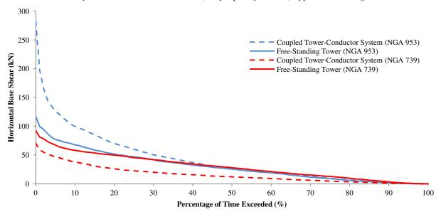
Figure 2: Persistence curve of horizontal base shear of Free-Standing Delta Guyed Tower and Coupled Delta Guyed Tower-Conductor System under NGA #953 record (low frequency content) and NGA #739 record (high frequency content) applied in longitudinal direction.
