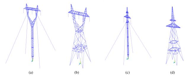
Figure 2. The 3-D view of Finite Element Models developed in ANSYS-APDL environment. (a) Delta Guyed tower, (b) Delta Self-supporting tower, (c) Mast Guyed tower, and (d) Mast Self-supporting tower.
