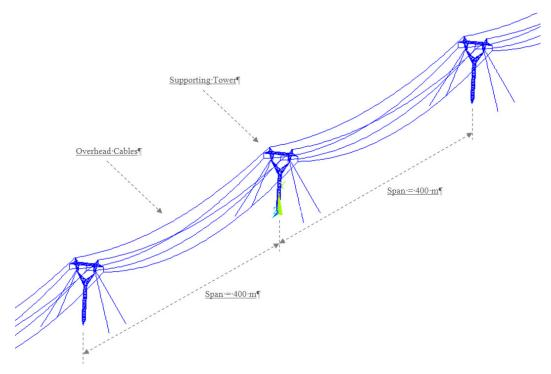
Figure 3. Perspective view of 315 kV HVAC straight transmission line segment
